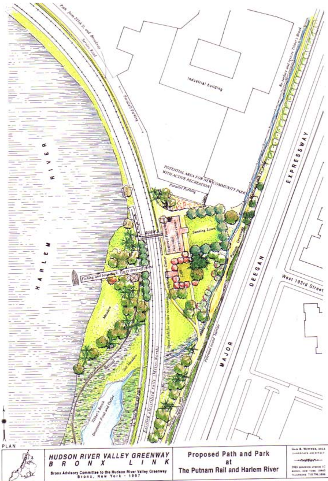
If Tibbetts Brook could be redirected down the Putnam Rail line, it could filter through wetlands before entering the Harlem River.
